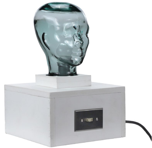
Light device used for assessing integrity of hood particulate blocking layer
