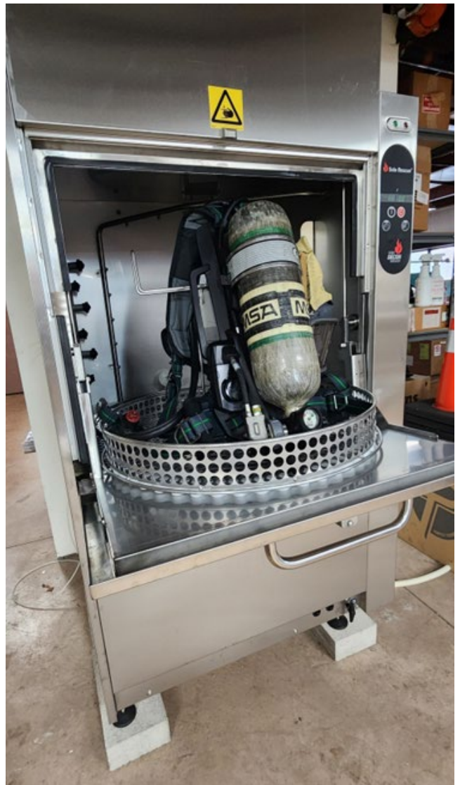
Special washing machine for SCBA and other PPE.
