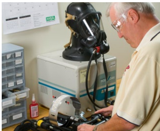
Authorized inspection and testing of SCBA at the fire department.
